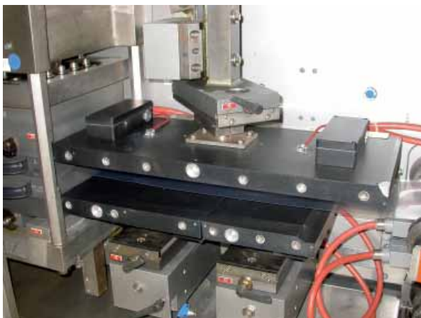
Heating Platens for Homogeneous Warm-Up of the PP Foil
